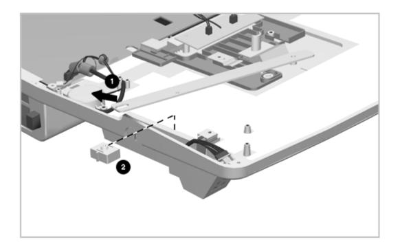
Figure 6-36. Removing the Docking Lever Slider
